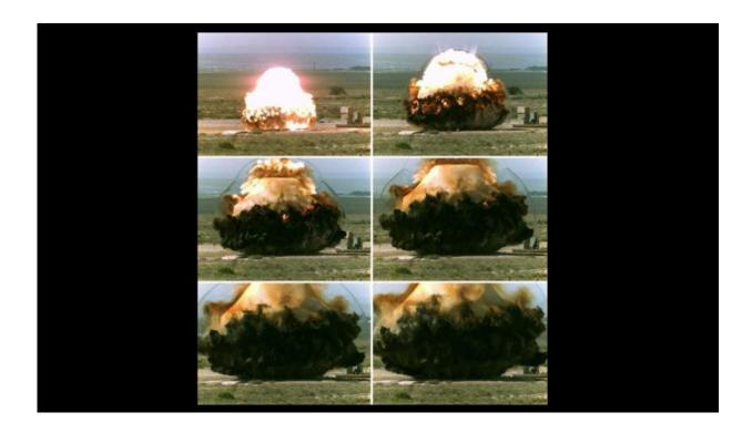
High-speed photographs of a controlled surface explosion at Kirtland Air Force Base in Albuquerque, New Mexico, similar to the explosions at White Sands Missile Range were used in a study of seismic signals to detect above-ground explosions. Credit: Defense Threat Reduction Agency (DTRA) Counter-WMD Test Support Division (CXT).
