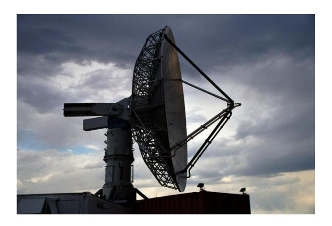
NCAR's portable S-Pol radar is one of the many instruments that will be deployed during the PECAN field campaign to help scientists better understand nighttime thunderstorms. Credit: ©UCAR
