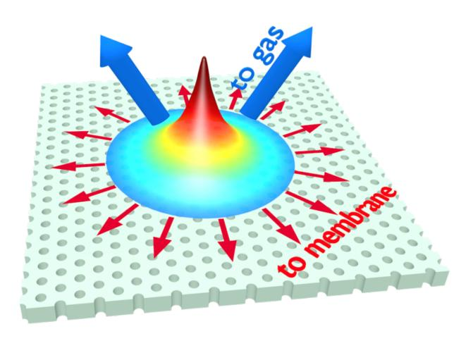
Once the laser beam hits the surface of a sample it starts to generate heat which diffuses along the membrane but also it diffuses to the ambient gas. That effect reduces the width of the temperature distribution in the photonic crystal
