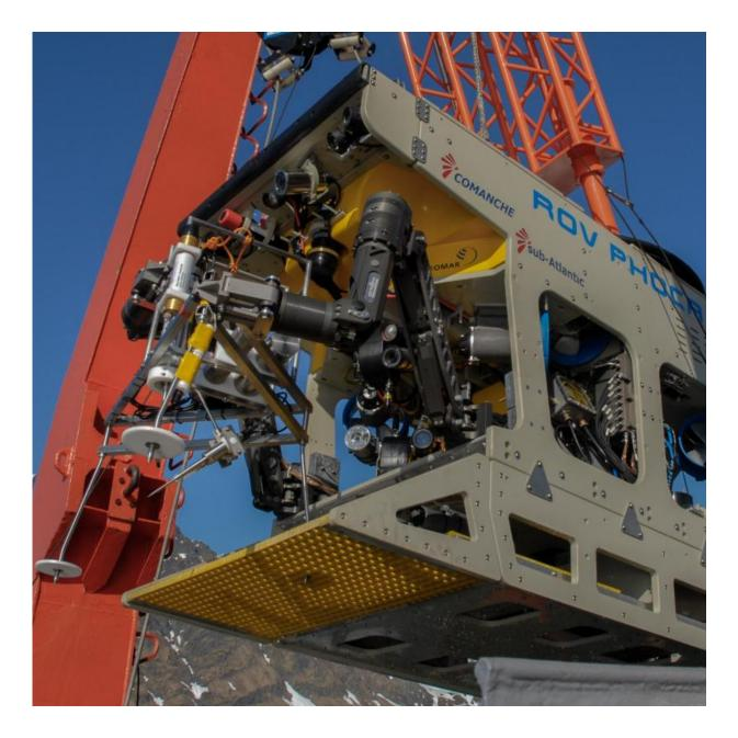
A photo of the Aquatic Eddy Covariance module on the GEOMAR ROV PHOCA remotely operated vehicle during deployment. Credit: Peter Linke, adapted from Rovelli et al. 2015
