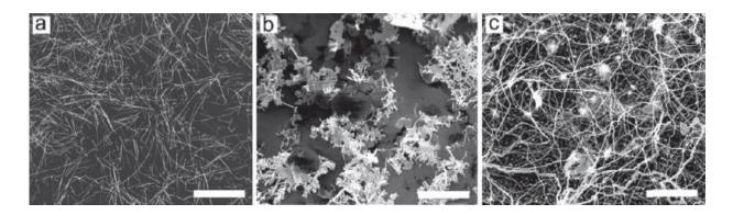
SEM images of various atomic switch networks consisting of silver nanowires. (a) and (b) lack reliable network density while (c) provides a tunable density of nanowires and spatially defined topology. The network is capable of emergent behavior and constant adaptation, traits of a brain-like complex system. Scale bar =  $50 \mu m$ . Credit: Demis, et al. ©2015 IOP Publishing
