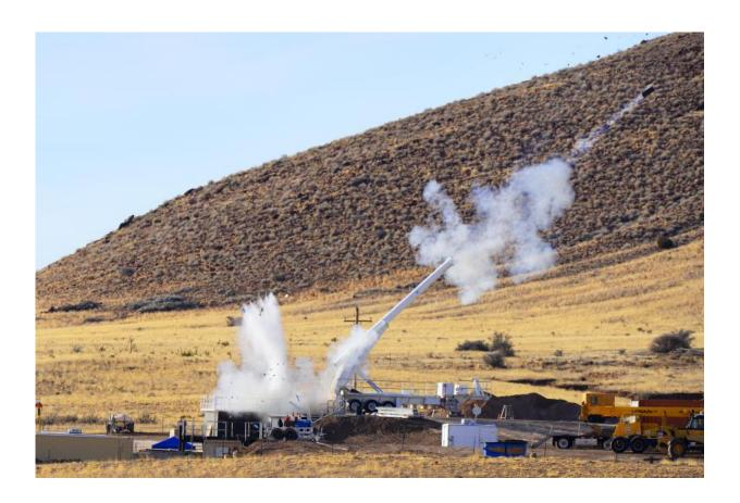
A test B61-12 nose assembly fired from Sandia National Laboratories' Davis gun splashes water from an 8-foot-deep pool as a 2,000-pound reaction mass sails into the air from the other end of the gun in a successful impact test at New Mexico Tech's Energetic Materials Research & Testing Center. The reaction mass eliminates the recoil load in the gun chassis during firing. Credit: Randy Montoya
