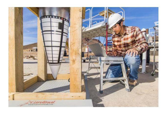
Tyler Keil, lead engineer for a test series using Sandia National Laboratories' Davis gun, performs a final diagnostics check on a data recorder for an impact test on the nose assembly of a mock B61-12. Data gathered from the test is helping analysts calibrate computer models. Credit: Randy Montoya
