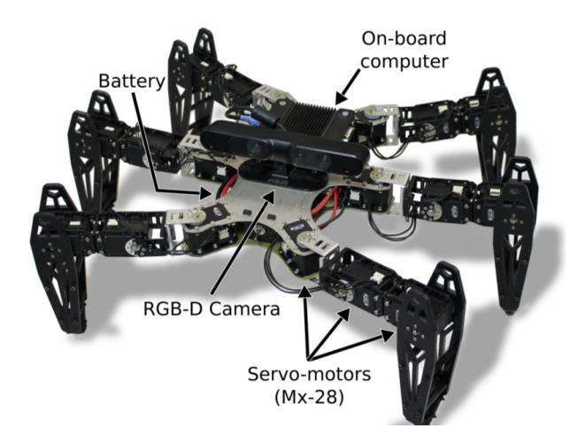
The undamaged hexapod robot. Credit: Antoine Cully/UPMC
