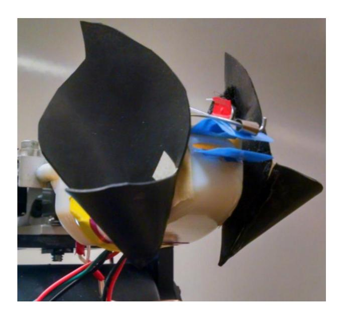
A new robot sonar prototype is inspired by the movable ears and noses that make up the echolocation systems of horseshoe bats. Credit: Philip Caspers/Virginia Tech
