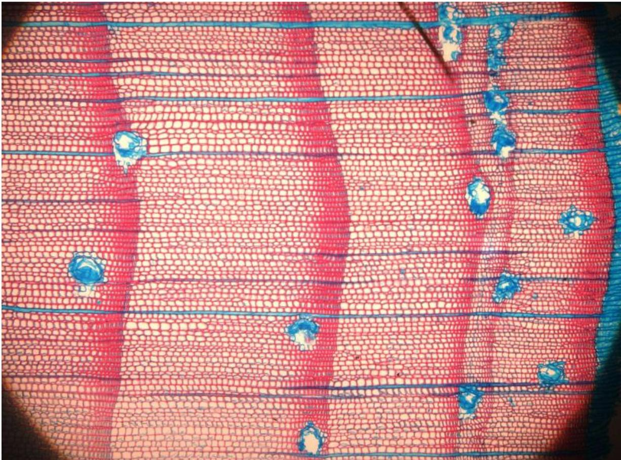
Optical microscope photo of a cross section of wood *Pinus pinaster*. Resin canals in blue color. Credit: Aída Rodríguez
