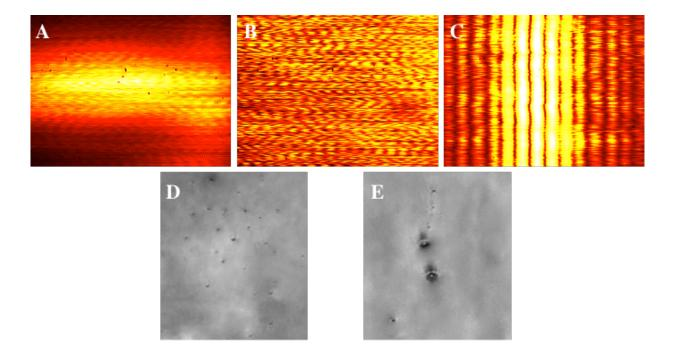
False color images of the interference pattern produced by a double slit for, (A), random Raman laser emission, (B), elastically scattered light and, (C), Helium-Neon laser emission. Strobe photography images of microcavitation bubbles forming, (D), before and, (E),\ after melanasomes are irradiated with 0.625 J/cm2 at 1064 nm. Credit: (A)-(C) Brett Hokr/ Texas A&M University, College Station, TX (D) and (E) Morgan Schmit/Optical Radiation Branch, Joint Base San Antonio, Fort Sam Houston, TX
