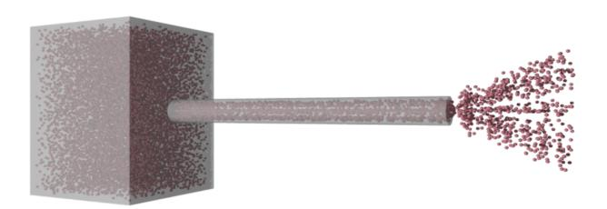
This schematic drawing shows a nanoscale faucet: a long cylindrical channel connected to a container of superfluid helium. When vacuum pressure is applied to one end of the faucet's opening -- a nanopore -- helium atoms (represented here as pink balls) flow through, and are collected and measured as they spread out. An incredibly sensitive detector is needed to register the hundredths of nanograms of helium that flow through each second. Credit: Adrian Del Maestro
