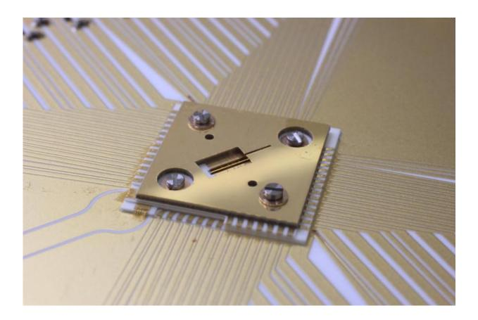
The scientists used this ion trap to create the new quantum states. Credit: ETH Zurich
