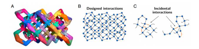
Controlled nucleation is essential for robust self-assembly. (A) An example 86-strand DNA-brick structure and (B) its associated connectivity graph. (C) Incidental interactions between dangling ends, shown in orange, lead to incorrect associations between fragments. Credit: (c) 2015 *PNAS*, DOI: 10.1073/pnas.1502210112
