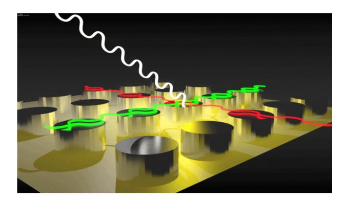
Magnetic nanoparticles arranged in arrays put a twist on light: depending on the distance between the nanoparticles, one frequency of light (visible to the human eye by its colour) resonates in one direction; in the other direction, light (induced by quantum effects in the magnetic material) is enhanced at a different wavelength. Credit: Aalto University
