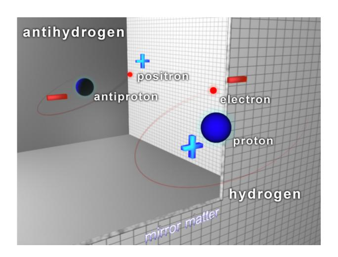
Antihydrogen consists of an antiproton and a positron. Credit: public domain
