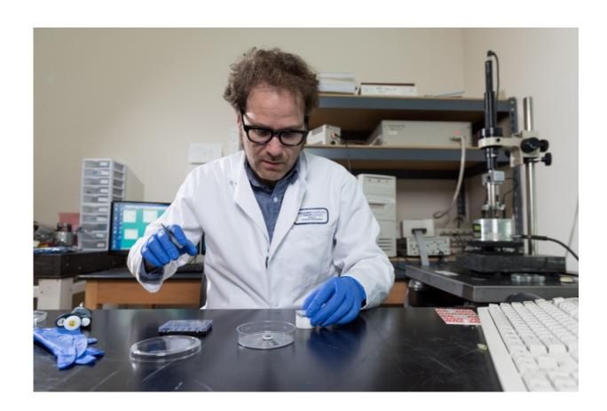
Georgia Tech postdoctoral researcher Isaac Gállego prepares a sample DNA nanostructure for imaging in an atomic force microscope. Credit: Rob Felt
