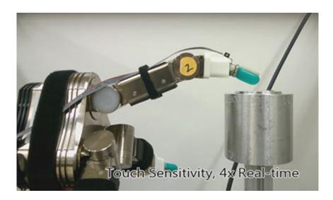
A robotic hand, or gripper, undergoes a NIST test to measure the contact force exerted by a robotic finger on an object. Credit: NIST
