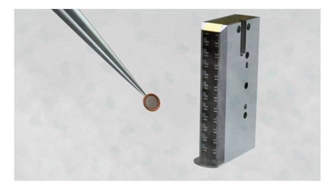
Carbon grid with frozen protein sample prepared for loading into cryo-electron microscope cartridge. Credit: Veronica Falconieri, NCI
