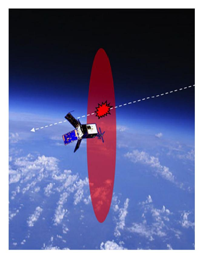
The Optical Orbital Debris Spotter is capable of detecting debris with sizes as
