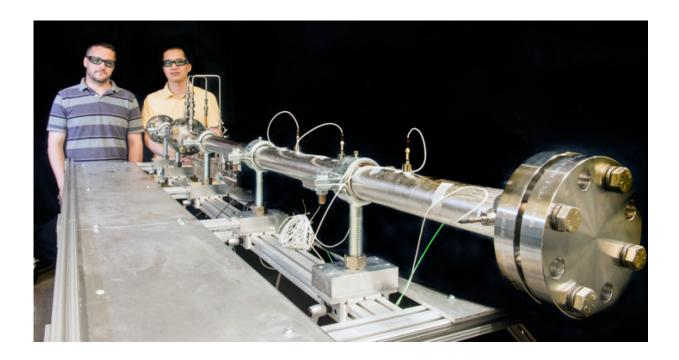
Kevin Douglass (left) and Haijun Liu with the initial experimental version of the shock tube.
