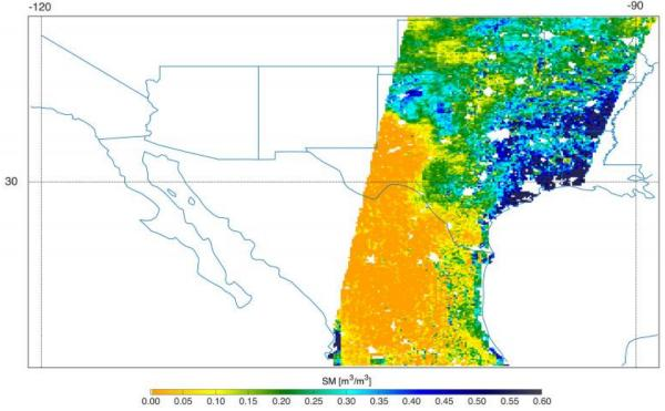
Southern U.S. SMAP soil moisture retrievals from April 27, 2015, when severe storms were affecting Texas. Top: radiometer data alone. Bottom: combined
