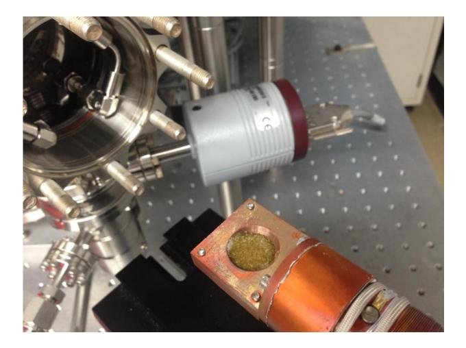
A salt sample, baked to a brownish color by radiation, after exposure to Europalike conditions. Credit: NASA/JPL-Caltech
