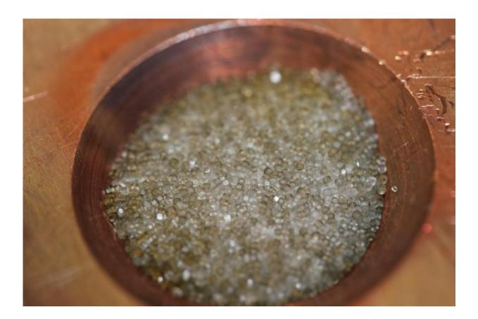
A close-up of salt grains discolored by radiation following exposure in a "Europain-a-can" test setup at JPL. Credit: NASA/JPL-Caltech
