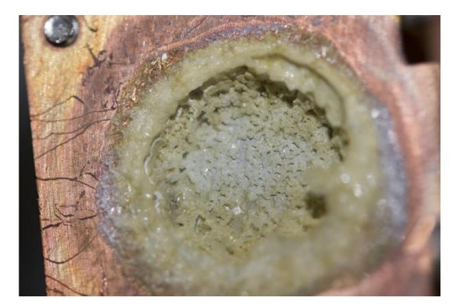
After tens of hours of exposure to Europa-like conditions, sodium chloride samples turned a yellowish-brown color. The color is spectrally similar to that of dark features on Europa imaged by NASA's Galileo spacecraft. Credit: NASA/JPL-Caltech
