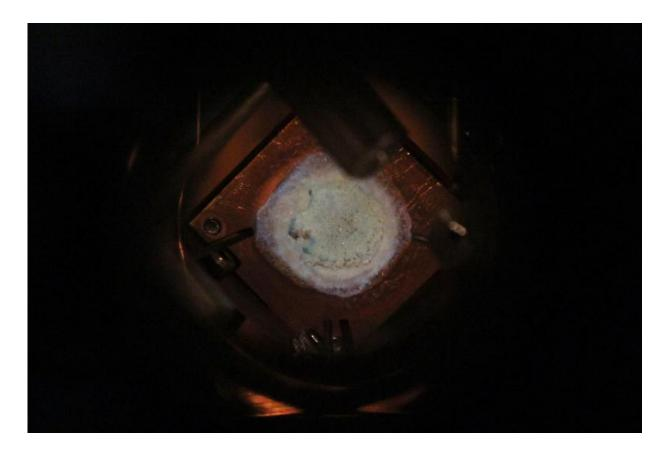
A salt sample inside a JPL test chamber is bathed in an eerie blue glow as an electron beam scans across it many times each second, delivering a powerful dose of radiation. Credit: NASA/JPL-Caltech
