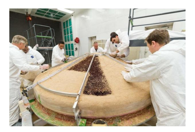
In this February 2015 scene from a clean room at Lockheed Martin Space Systems, Denver, specialists are building the heat shield to protect NASA's InSight spacecraft when it is speeding through the Martian atmosphere. Credit: NASA/JPL-Caltech/Lockheed Martin
