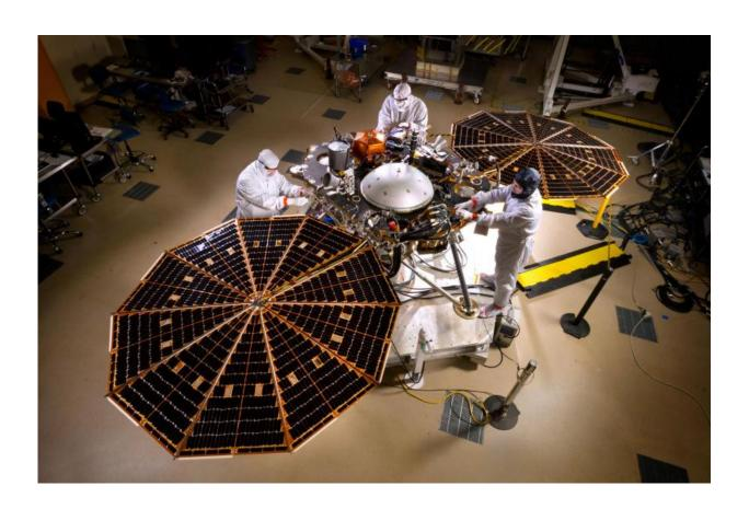
The solar arrays on NASA's InSight lander are deployed in this test inside a clean room at Lockheed Martin Space Systems, Denver. This configuration is how the spacecraft will look on the surface of Mars. The image was taken on April 30, 2015. Credit: NASA/JPL-Caltech/Lockheed Martin
