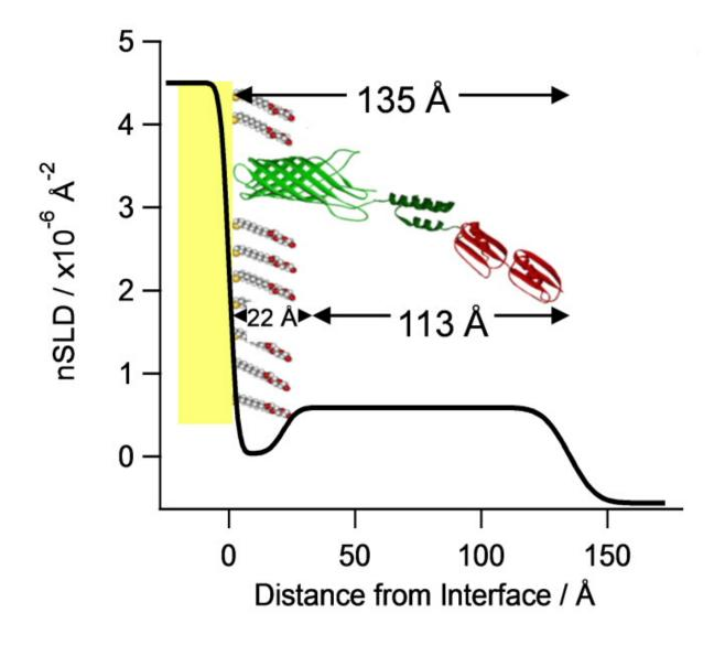
A 13.5 nm thick engineered-monolayer that self-assembles on gold surfaces, captures IgG (antibody) with high affinity in a defined orientation and specifically recognises the influenza A nucleoprotein.
