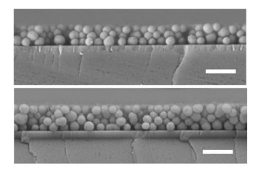
Electron micrographs of cross-sections of films made from nano particles of polydopamine. The thickness of the layers and density of particles determines how light interacts with the particles, and therefore the color of the film. The top film created a red hue, the bottom green. Credit: UC San Diego/University of Akron
