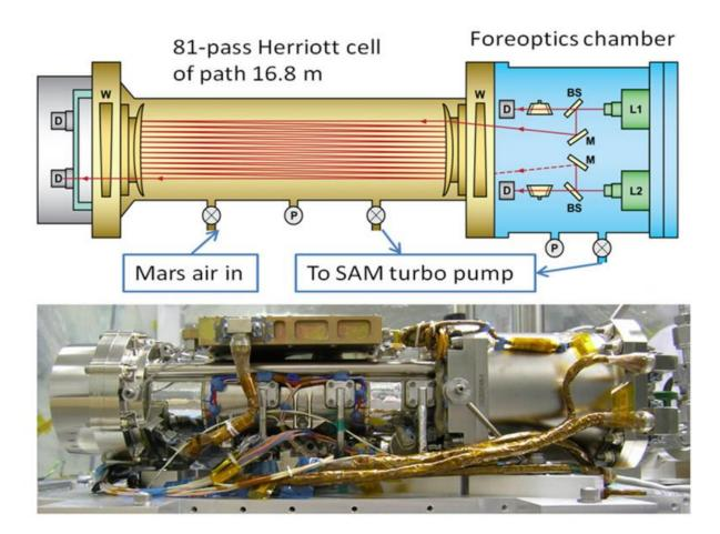
The Tunable Laser Spectrometer on NASA's Curiosity Mars Rover. The foreoptics chamber contains a small amount of methane for calibration purpose. Credit: NASA/JPL
