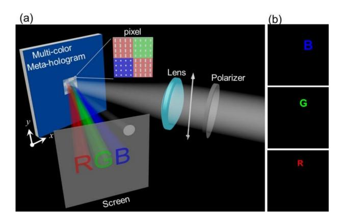
The multicolor meta-hologram is made of a pixel array consisting of aluminum nanorods of different lengths that produce different colors of light. Credit: Huang, et al. ©2015 American Chemical Society
