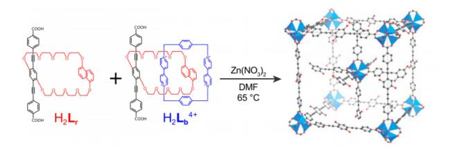
MOF-2000 is a periodic framework harboring controlled component heterogeneity. Chemical structures of organic struts H2Lr and H2Lb4+ incorporated in MOF-2000 (Methods Summary), and the MOF-2000 crystal structure [key: carbon, black; oxygen, red; Zn4O(CO2)6 polyhedra, blue; all hydrogen atoms have been omitted for clarity]. Credit: (c) 2015 *PNAS*, 10.1073/pnas.1416417112
