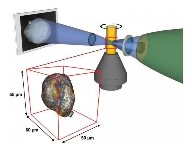
SSRL X-rays are focused to illuminate a small sample of catalysts inside a movable cylindrical holder. A lens magnifies the resulting sample image onto a screen, a CCD camera captures the 2-D image, and software is used to reconstruct a 3-D image of the single catalyst particle from a series of these 2-D images. Credit: Florian Meirer/Utrecht University
