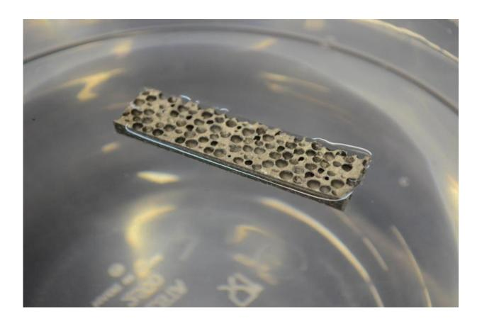
The first metal matrix syntactic foam is so light it can float, strong enough to withstand the rigors of a marine environment, and resistant to heat, which makes it a candidate for automakers seeking to shed weight to improve fuel economy. The composite was the work of NYU Polytechnic School of Engineering Professor Nikhil Gupta and Deep Springs Technology (DST) in collaboration with the U.S. Army Research Laboratory. Credit: NYU Polytechnic School of Engineering
