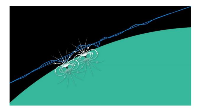
Schematic magnetic field lines (in white) from magnetized crustal rocks on Mercury. As the MESSENGER spacecraft passed over a region of crustal magnetization, its Magnetometer measured small variations in the magnetic field (blue line). Because the signals are small, they were observed only when MESSENGER was close to the planet. Credit: NASA, University of British Columbia
