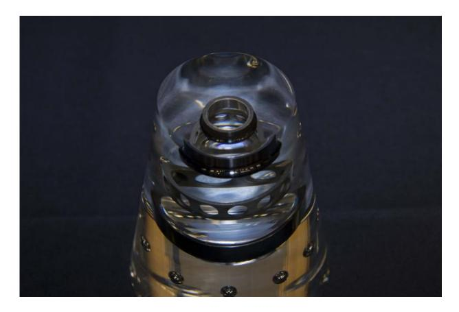
Bearing for a satellite mechanism, displayed in glass, lubricated with molybdenum disulphide. This widely used solid lubricant can withstand prolonged vacuum conditions. Credit: ESA–A. Le Floc'h
