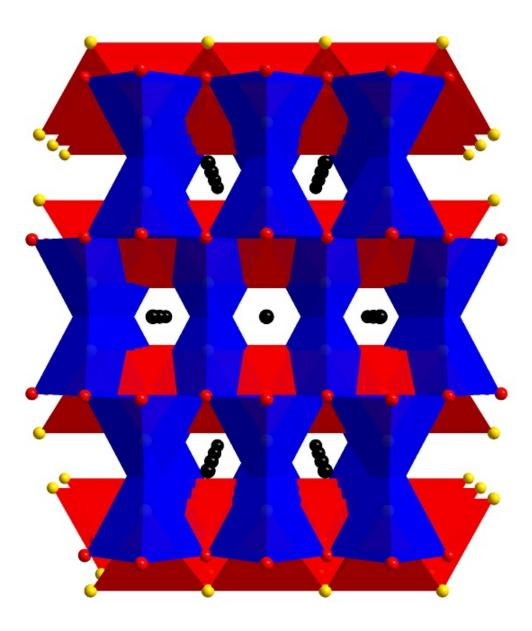
Collapsed tetragonal crystal structure of NaFe2As2, with arsenic (As) atoms in a 5-fold coordination, courtesy of Alexander Goncharov. Sodium (Na) is represented by the black balls, iron (Fe) by the red balls, and arsenic (As) by the yellow balls. Courtesy of Alexander Goncharov. Credit: Alexander Goncharov
