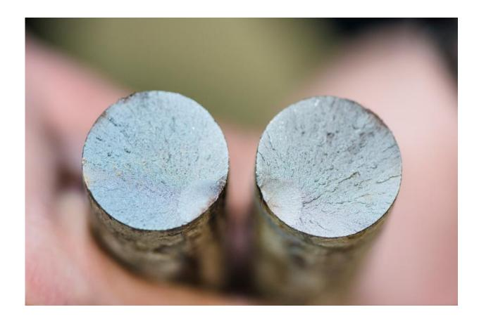
This pre-stressing steel sample broke during the fatigue test. Credit: Gorczany
