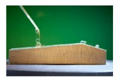
Water droplets can be moved in different directions by changing the temperature of the textured block
