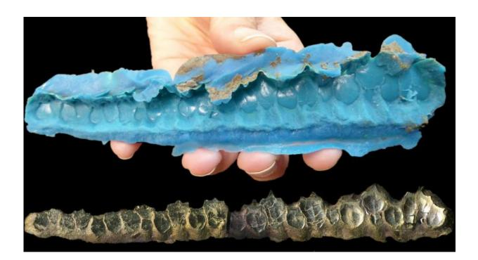
A high fidelity rubber mold of hadrosaurid dinosaur teeth, with a gold coated replica for measurement of roughness of the tooth surfaces. The surfaces have scratches that were created as the dinosaur fed on vegetation 67 million years ago, and measuring the roughness can reveal what kind of food they ate. The original teeth are too large to transport to the instrument that measures roughness. Credit: University of Leicester
