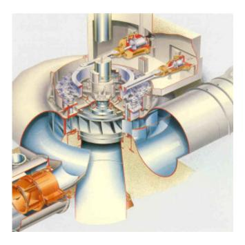
A drawing showing the essential elements of a Francis turbine, one of the most common hydropower turbines in Norway. Credit: Kværner
