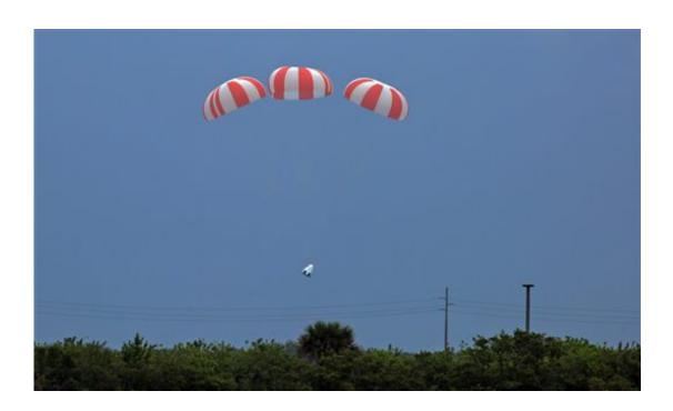
SpaceX's Dragon crew capsule parachutes deploy Wednesday, May 6, 2015 from Cape Canaveral, Fla. SpaceX fired the mock-up capsule to test the new, super-streamlined launch escape system for astronauts. (Red Huber/Orlando Sentinel via AP)
