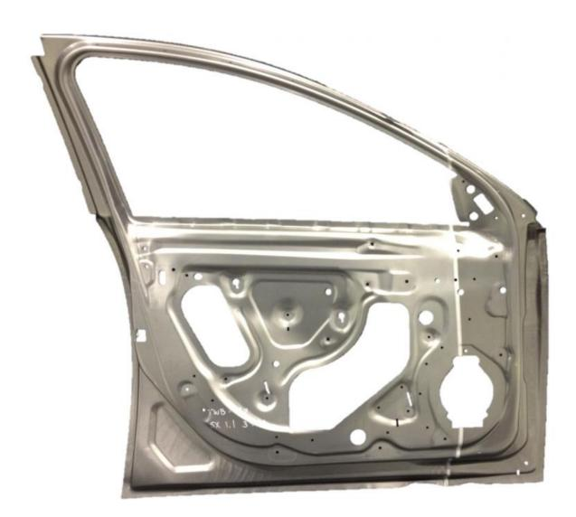
PNNL's process joins (white line) a thicker gauge of aluminum near the door hinge, where additional strength is needed, to a thinner gauge used throughout
