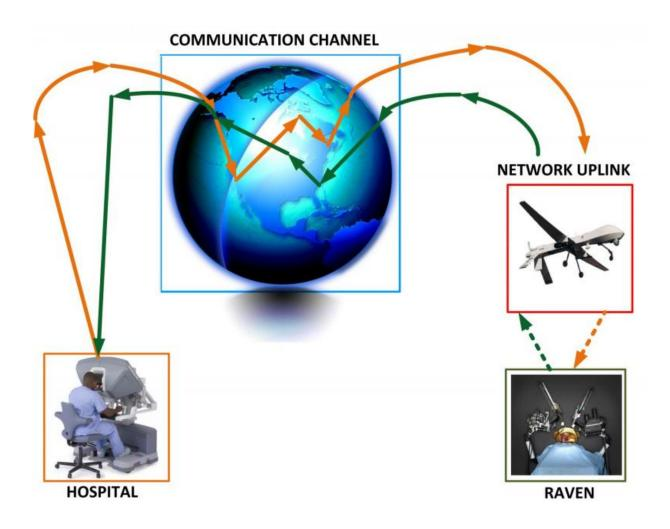
In future telerobotic procedures, the last communication link may a wireless uplink (dotted lines) to a drone or satellite that is more easily hacked than preestablished network connections (solid lines.) Credit: University of Washington
