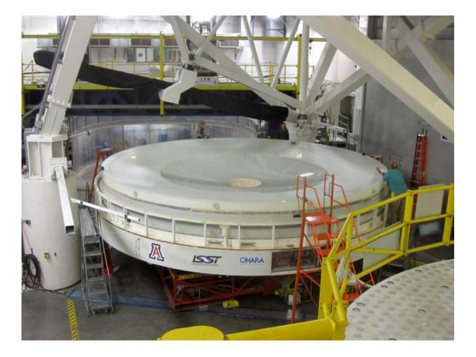
Measuring 27 feet in diameter, the LSST mirror rests on the polishing table in the UA's Richard F. Caris Mirror Lab. It's the only mirror in the world that combines a large primary mirror and a smaller tertiary mirror in one piece. Credit: Mirror Lab/LSST Corp.
