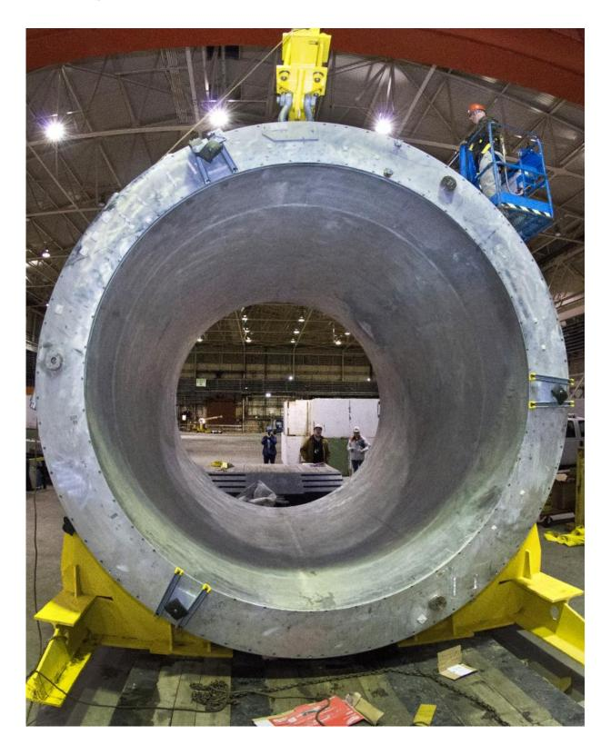
Engineers prepare to move the 20-ton solenoid into its new home at Brookhaven Lab.
