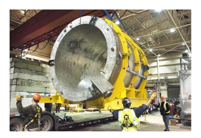
The massive, just-delivered magnet leaves the truck inside Brookhaven's Superconducting Magnet Division.
