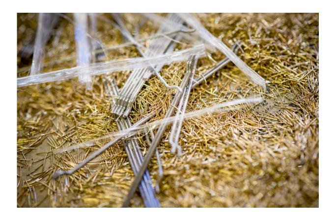
In order to make the shotcrete more robust, RUB engineers add steel fibres into the mixture. Credit: RUBIN, photo: Gorczany
