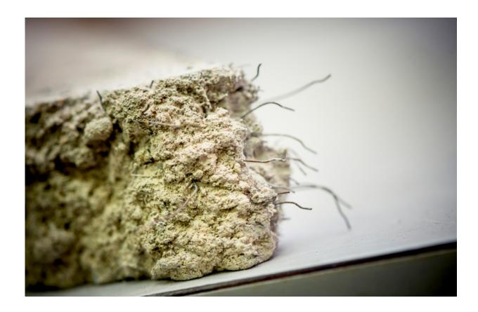
Steel and synthetic fibres make the new shotcrete more robust. Credit: RUBIN, photo: Gorczany
