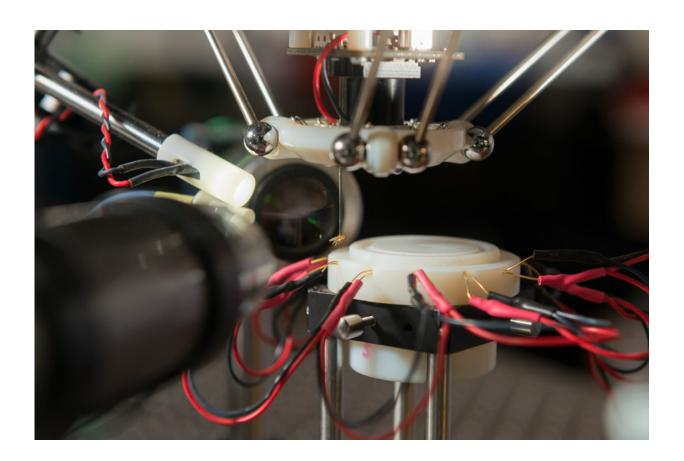
A fruit fly hangs unharmed at the end of the robot's suction tube. The robot uses machine vision to inspect and analyze the captured fly. Credit: L.A. Cicero
