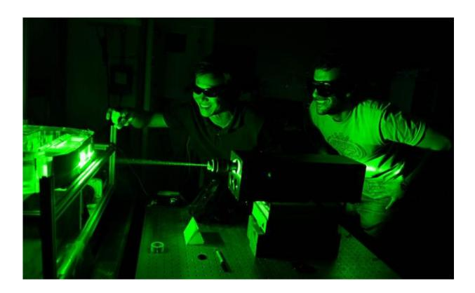
James Liao and Otar Akanyeti from UF's Whitney Laboratory use lasers to track the flow of water over a model of a fish. Learning about a fish's "sixth sense" could help scientists understand human systems such as those in the inner ear.
