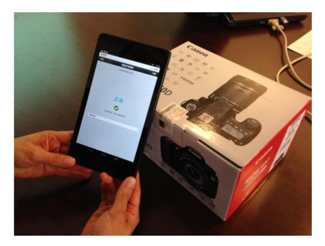
A Verayo chip is integrated into a label on a Canon camera box. When scanned with a mobile device, a check mark signifies that the chip is authentic. Credit: Srini Devadas
