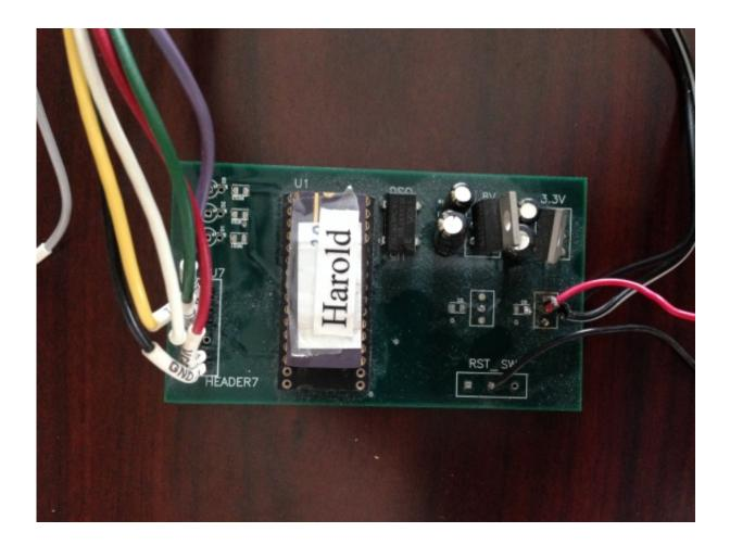
One of Devadas's early PUF-enabled circuits, labeled with the name "Harold." When this circuit was scanned with a custom reader, its name would pop up on a computer screen. Credit: Srini Devadas
