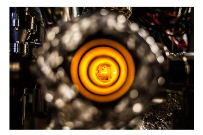
Sodium atoms diffuse out of an oven to form an atomic beam, which is then slowed and trapped using laser light. Credit: Jose-Luis Olivares/MIT
