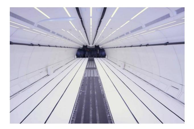
An inside view of the refitted Airbus A310 aircraft. Although the aircraft can weigh up to 157 tonnes, skilled pilots angle its nose 50° upwards to create brief periods of weightlessness. At the top of each curve, the forces on the passengers and objects inside cancel each other out, causing everything to float in weightlessness. Credit: Novespace
