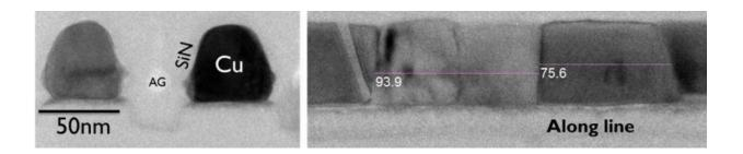
Figure TEM section of copper etched lines encapsulated by SiN cap layer.
