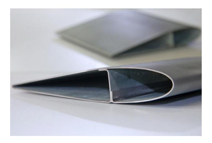
Technology demonstrator: formed from a 1.0 mm steel sheet and featuring integrated, folded reinforcement, the rotor blade was given its final shape with the help of an oil-water mixture. Credit: Fraunhofer IWU
